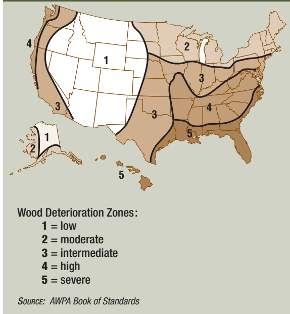
Figure 1: Wood Deterioration Zones
